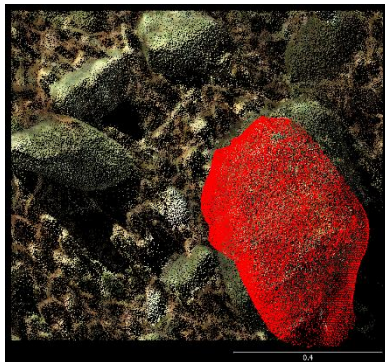
Figure 10 Position of point clouds after initial transformation, red – aligned point cloud
