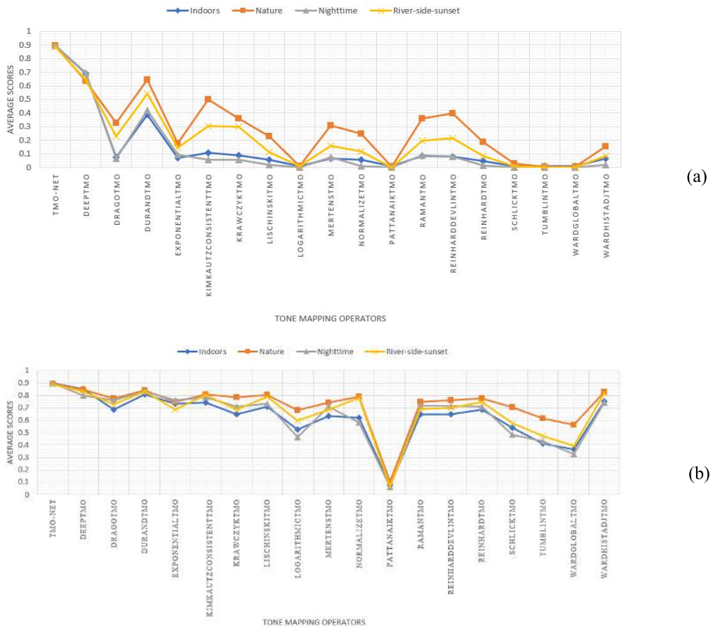
FIGURE 9. Performance comparison of selected operators on scene categories of the LVZ-HDR benchmark dataset. plot (a) shows the average naturalness score while plot (b) shows the average TMQI-Q score per scene category of the dataset. It can be observed that TMO-Net exhibits better performance index across all scene categories.
