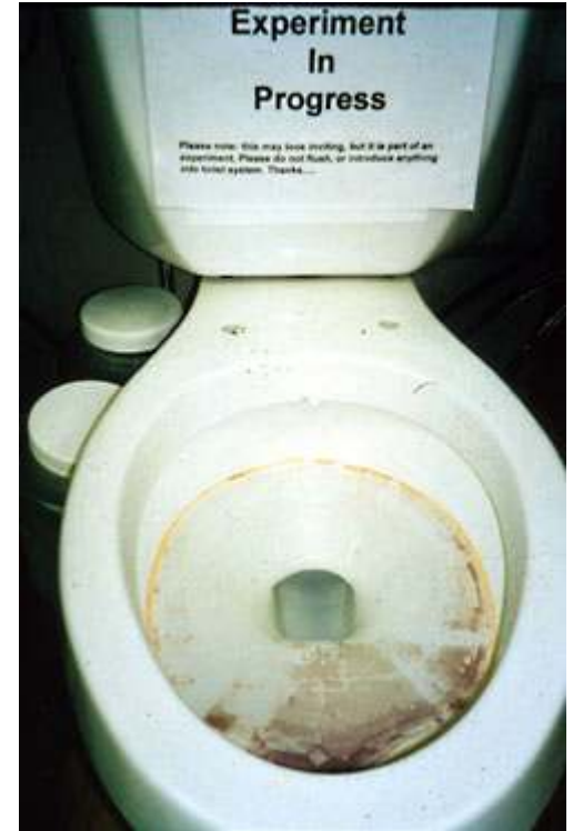
Biofilm in toilet
