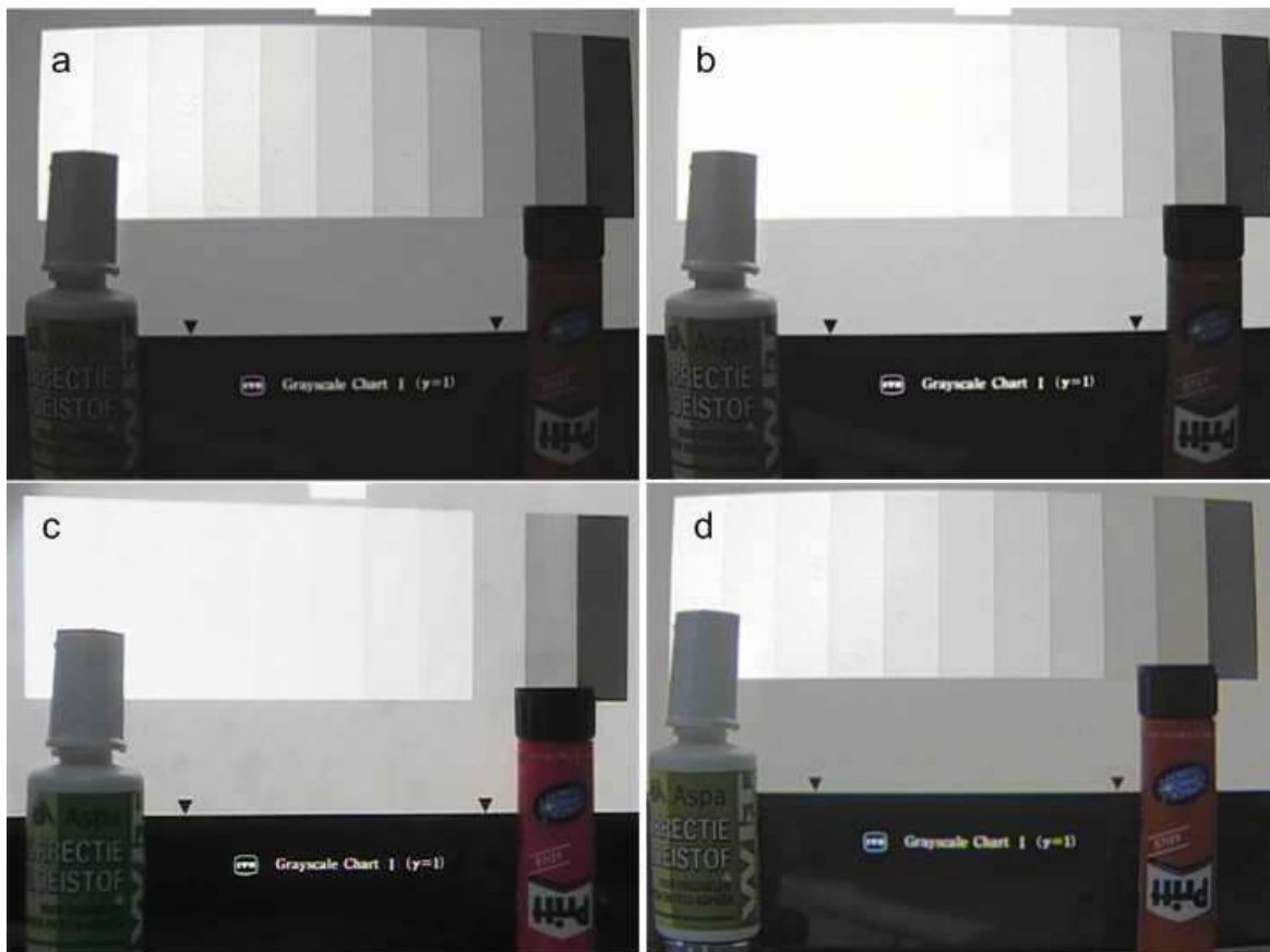
Fig. 11. Results: (a) standard camera image, (b) smart extended range Gamma, (c) method from the [4], (d) our method ( \alpha=0.5 ).
