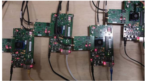
Figure 13: Each AP is a latest WARP v3 Kit with FMC-RF-2X245 module to enable 4 radios. Antennas are placed at the dedicated AP positions with low loss LMR-400 cables.
