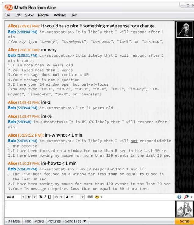
Figure 7: IM Autostatus. Demonstration of various explanations from an IM responsiveness prediction plugin that uses a decision tree to predict when a buddy would respond.
