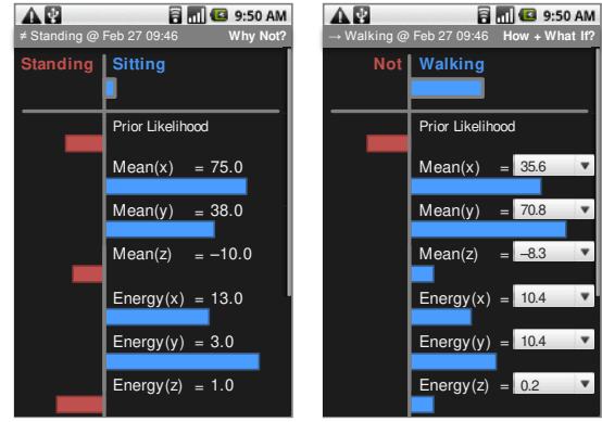
Figure 6: Why Not (Left), and How To + What If (Right) explanations for a mobile phone physical activity recognition application using accelerometer data trained with a naïve Bayes classifier. The application has inferred that the user is Sitting .
