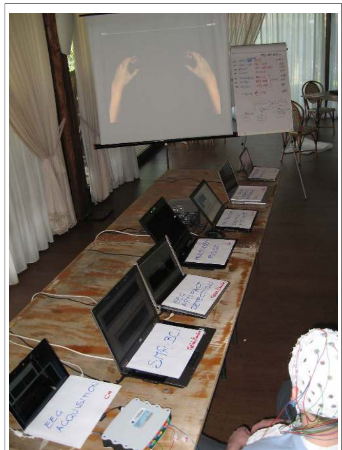
FIGURE 7 | This picture was taken during the demonstration of the proof of concept. Here, all connected computers, forming a demo hybrid BCI, are visible. The first was used for data acquisition, running the SignalServer, and the next two were used to build an SMR BCI and an artifact detection. Laptop number four was a very simple implementation of fusion. Laptops five and seven formed together the visual feedback, presented on the screen (control interface and feedback application). The sixth laptop showed an additional operator feedback which was not presented to the subject.
