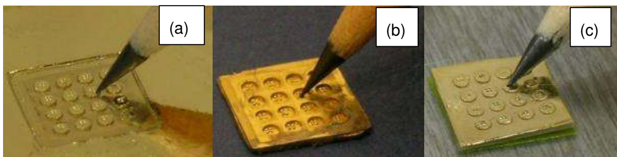
Figure 4.12: (a) PC template fabricated by lithography and milling; (b), electroplated nickel tool; (c), and HDPE foils embossed from the nickel tool.
