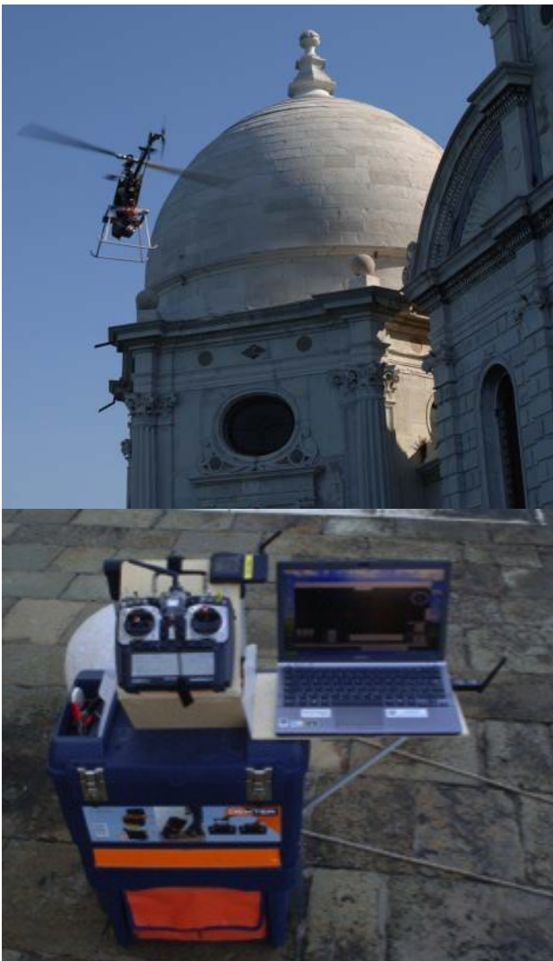
Figure 5. the Align Trex helicopter, equipped with GPS and the Sony Nex camera and its ground control
