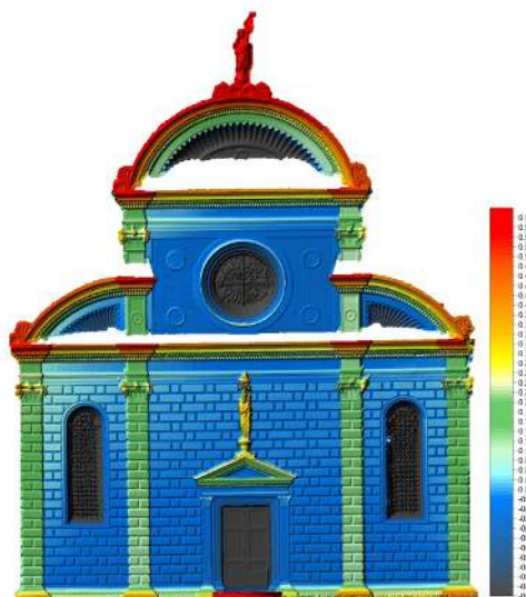
Figure 4. DSM of the facade of the church with “shadow” zone due to entablatures
