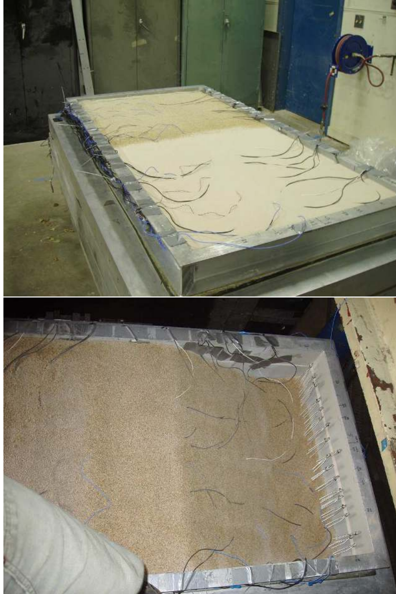
Figure 3.1: Photos of physical models: a flat ground configuration (top) and a single slope with angle of 30^\circ (bottom)
