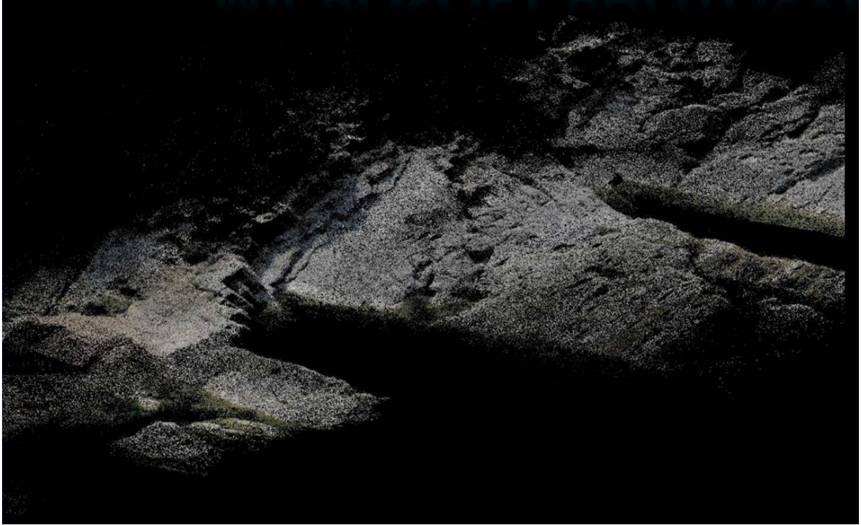
Figure 7. Oblique view of a section of the Pedernales Falls research area georeferenced point cloud. The length of this point cloud area is approximately 200 meters. The large linear black areas are deep water.
