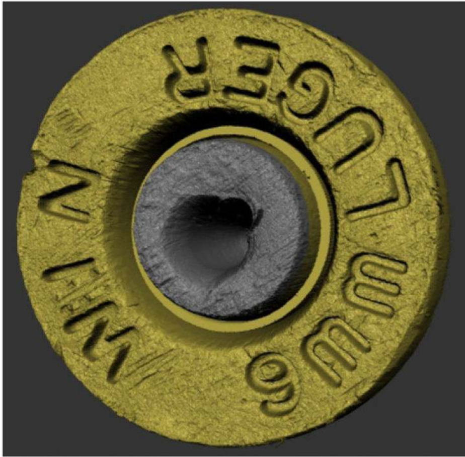
Figure 13. Topography image of a fired cartridge case obtained with a method closely related to CSI (reprinted with permission) [35].
