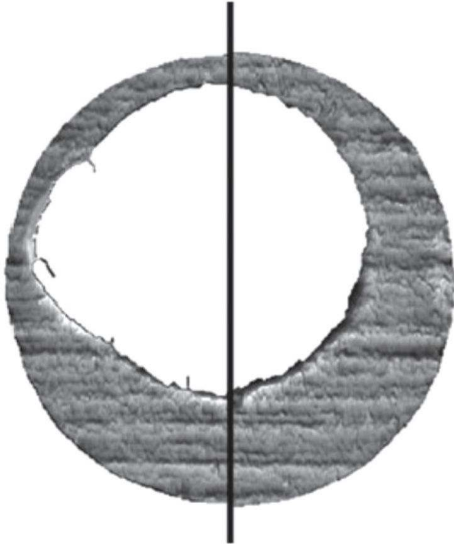
Figure 34. Side by side comparison of two breech face impressions from the same Sig Sauer P226 9 mm Luger firearm obtained with confocal microscopy by Riva and Champod (©2014 American Academy of Forensic Sciences, reproduced with permission of John Wiley and Sons).
