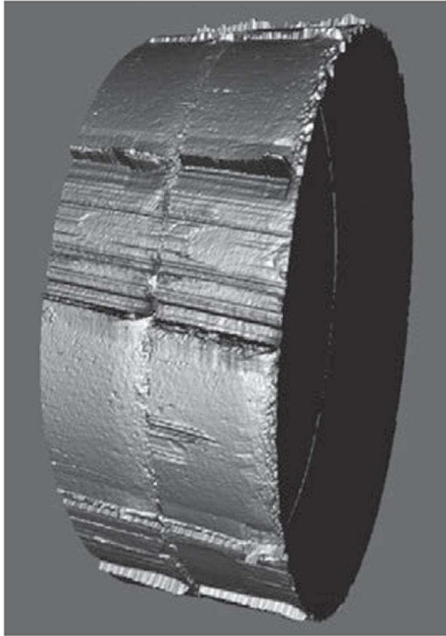
Figure 10. Topography image of 360° bands of two fired 9 mm caliber bullets obtained with disk scanning confocal microscopy. For each image, the system captured and stitched 1.6 mm × 1.6 mm areas while rotating and translating the bullet (courtesy of Ultra Electronics Forensic Technology, Inc. [3]).
