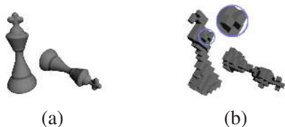
Fig. 3. The digital reconstruction (b) of an r -regular object (a) may not be well-composed, i.e. its surface may not be a 2D manifold as can be seen in the magnification.
