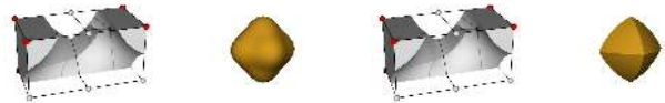
Fig. 15. Left: Examples of trilinear interpolation without blending. Right: The same examples with with C^\infty -blending.
