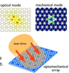
and phonons can tunnel between different sites in this array. Their effective interaction can be modulated by the drive laser frequency, intensity, and phase.
