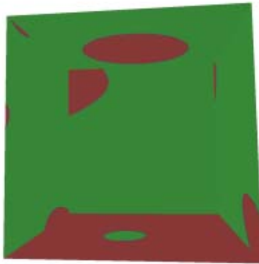
FIGURE 9: The boundary box and the flow patterns on the faces of the box. The inflow faces are shown in red, the outflow faces in green and the faces with tangential flow are shown in blue.
