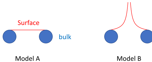
Figure 3. The energy contour of surface states for Model A (left panel) and Model B (right panel). The blue areas stand for bulk projections (enclosing WNs) and red lines are for surface states. That Fermi arcs in Model B do not connect is visible.
