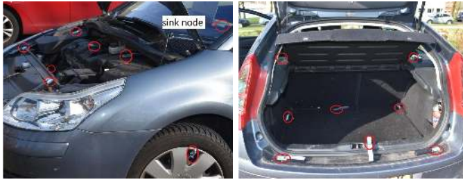
Fig. 6. Experimental testbed with 30 JN5168 [33] wireless sensor nodes distributed over a car.
