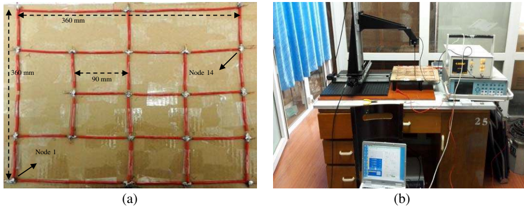
Figure 18. Experimental model and lab test. (a) Illustration of 5 \times 5 square grid made of copper wires. The dimensions of the grid are 360 \text{ mm} \times 360 \text{ mm} and mesh spacing is 90 \text{ mm} . DC current is injected at Node 1 and received from Node 14. (b) Lab test.
