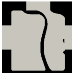
Figure 5.10: Example of an undesirable optimized design for the pump problem with enforced pressure drop.
