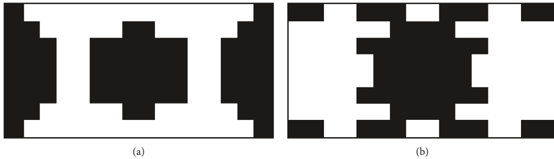
FIGURE 8: The optimal layouts of CLD treatment. (a) f = [0, 100] Hz and (b) f = [100, 1000] Hz.
