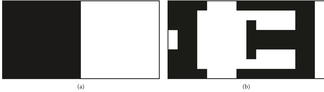
FIGURE 3: The optimal layouts of CLD treatment. (a) f = [0, 100] Hz and (b) f = [100, 1000] Hz.
