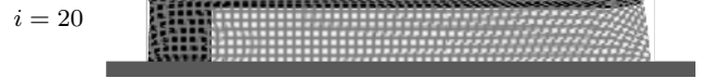
Fig. 8: Displacement plot of the cantilever example with a mesh resolution of n = 300 \times 40 = 12000 elements.
