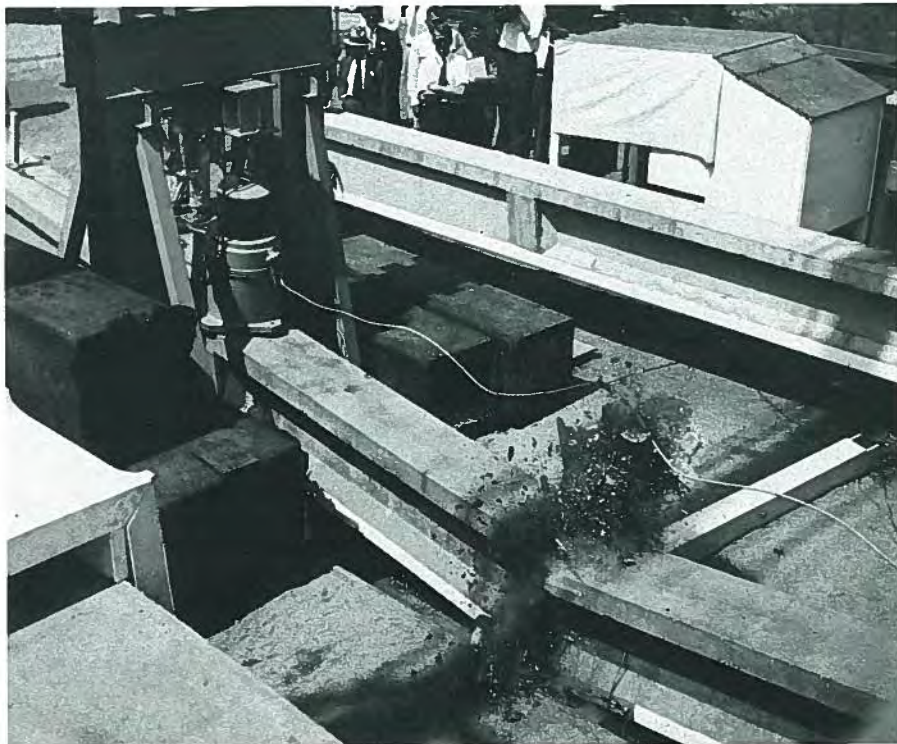
Fig. 40. Explosive failure (with top flange failing in compression) of 40-ft (12.2 m) girder (P-40) using unbonded tendons (Austin Company tests).
