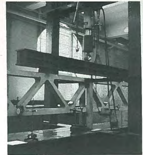
Fig. 25. Prototype truss undergoing testing in laboratory.
