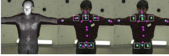
Figure 4: Regressing detection target 3D positions. (Left) The template model is aligned with target object; (Mid.) The torso joints of the template model (magenta) have discrepancy from the joint definitions of 3D keypoint detection (cyan); (Right) The newly regressed target locations (green) are more consistent with 3D keypoint detections.
