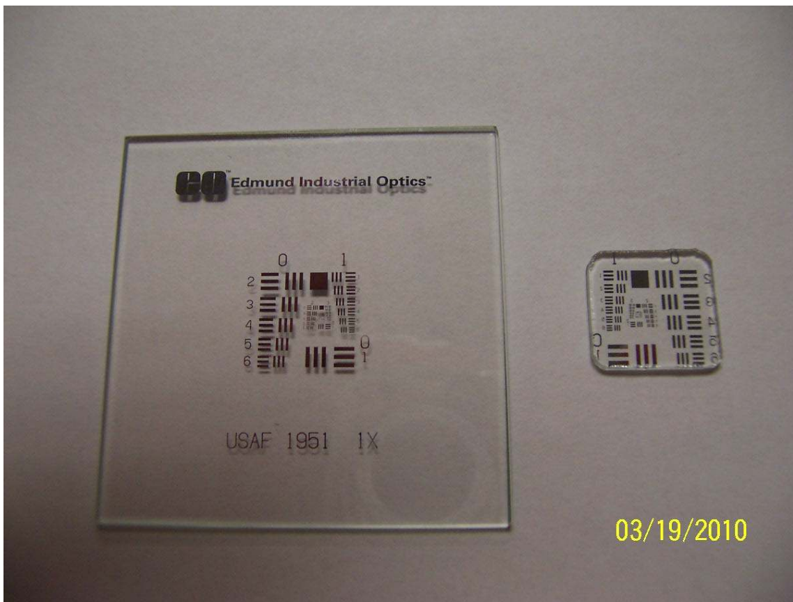
Figure 4.1 USAF 1951 1X Resolution Target. A 2" x 2" resolution target (left) and cut down chip for emplacement on TIR prism face (placed in glycerin for optical path continuity)
