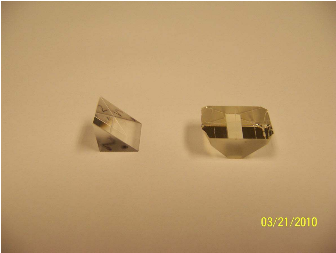
Figure 3.1 TIR Prism. On the left is a 12.7mm (hypotenuse 17.5mm) right angle BK7 glass ( n = 1.517 ) unit, Melles Griot Part Number #01 PRS 011. (Unit 2) At right is a truncated 15.00 mm (Hypotenuse 21.00mm) right angle SFL11 glass ( n = 1.785 ) unit, made from Edmund part number NT45-950- Scribelines for prism alignment are barely visible on the upfacing hypotenuse of the SFL11 unit.
