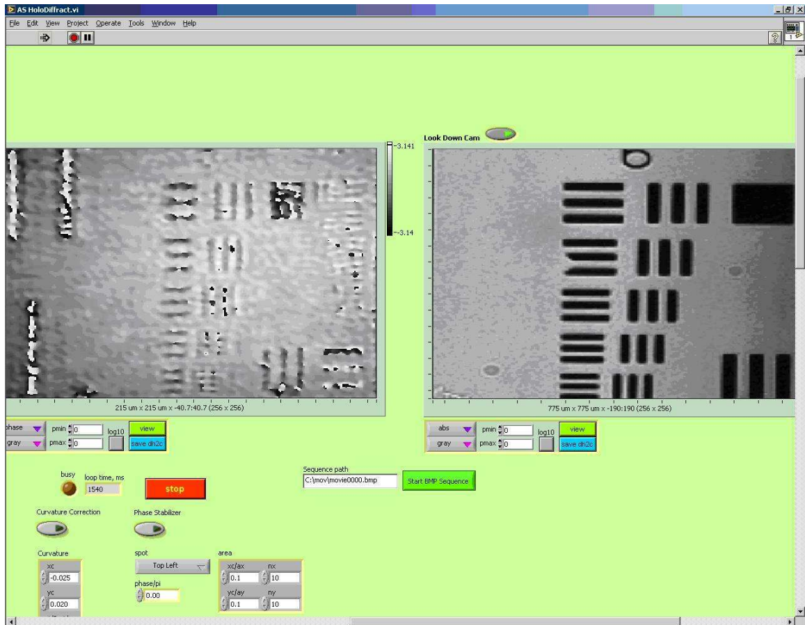
Figure 4.7 AS HoloDiffract.vi RT calibration run; Operators Console. Phase image of RT on left, LookDown camera feed on right. Tilt compression in phase image is in x-direction. Operation in this configuration allows the operator real-time simultaneous viewing of phase image and Lookdown direct image. Note movie sequence control <Start BMP Sequence> below image windows. The curvature correction and phase stabilizer controls for software compensation are also visible at bottom left.
