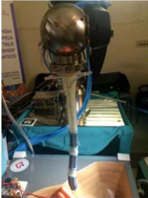
Fig. 3 Three-segment STIFF-FLOP arm with embedded sensors, connected to the SCHUNK robot
