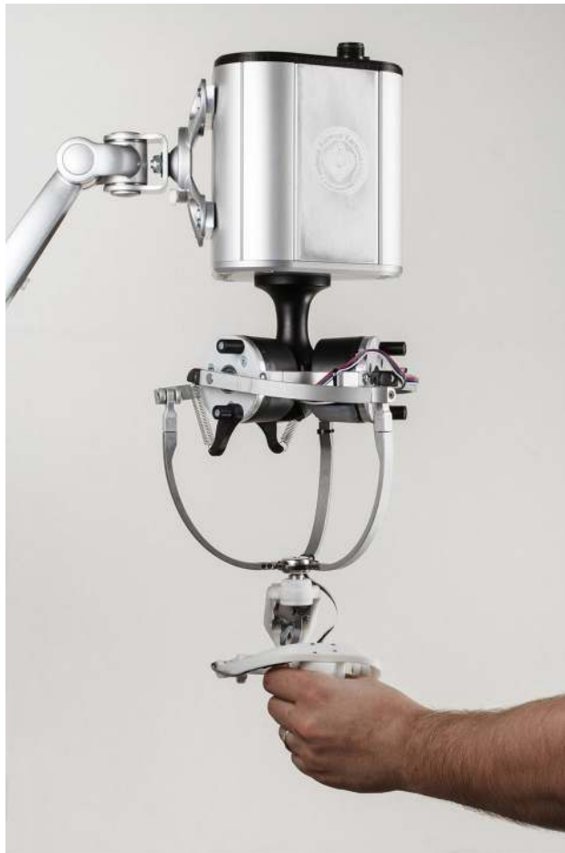
Fig. 4 Six degrees of freedom (DoF) haptic input device, based on a Delta robot design
