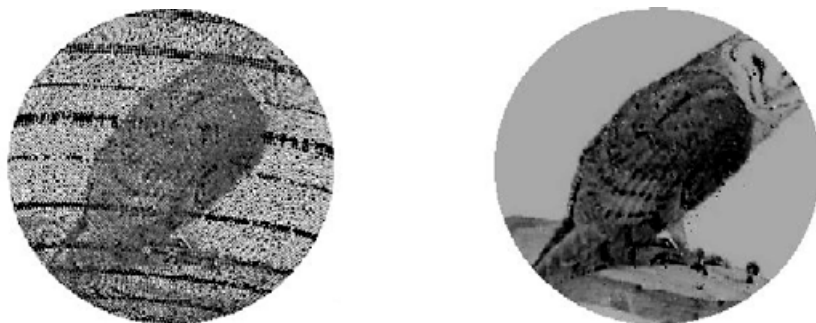
Figure 6.5. The image on the right is the denoised and inpainted result from the left.
