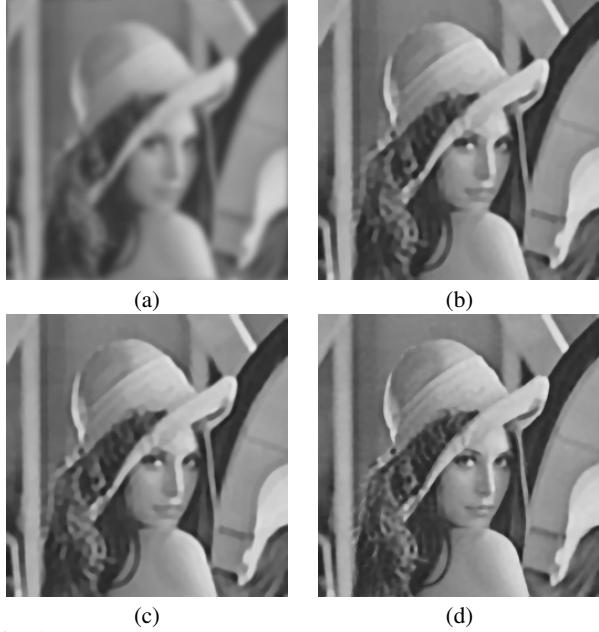
Fig. 1. (a) Image degraded by a Gaussian shaped PSF with variance 9 and Gaussian noise of variance 0.16 (BSNR=40dB), (b) Restored image using ALG1 (ISNR = 4.84dB), (c) Restored image using ALG2 (ISNR = 4.64dB), (d) Restored image using ALG1-True (ISNR = 6.95dB).
