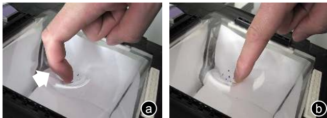
Figure 22: (a) A hooked finger accidentally touching the opposite side of the bowl. (b) Switching back to a straight finger posture avoids the issue at the expense of the increased error.
