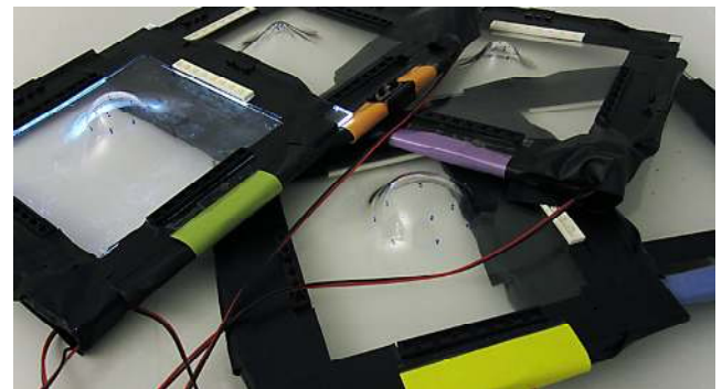
Figure 10: We implement different curvatures by using replaceable top units.
