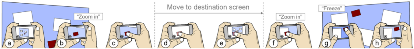
Figure 7. Dragging an object with the updated Touch Projector: (a) the user aims at a display (b) causing the device to automatically zoom in. (c) This allows the user to touch the red target object and (d) hold it while turning the device towards the other display. (e) Once the device detects the secondary display, (f) it zooms in again. (g) Pushing the freeze button with the thumb of the non-dominant hand causes the live camera image to pause for precise manipulation. (h) Lifting the finger releases the object.
