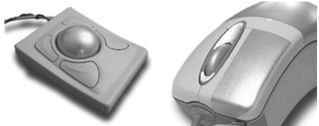
Fig. 1 Left: The TouchTrackball (a modified Kensington Expert Mouse) senses when the user touches the ball. Right: The Scrolling TouchMouse (a modified Microsoft IntelliMouse Pro) senses when the user is holding the mouse by detecting touch in the combined palm/thumb areas. It can also sense when the user touches the wheel, the areas immediately above and below the wheel, or the left mouse button.
