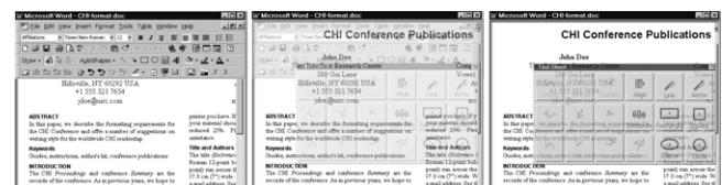
Fig. 4 When the user touches the trackball, the ToolGlass fades in quickly; the toolbars simultaneously fade out.
