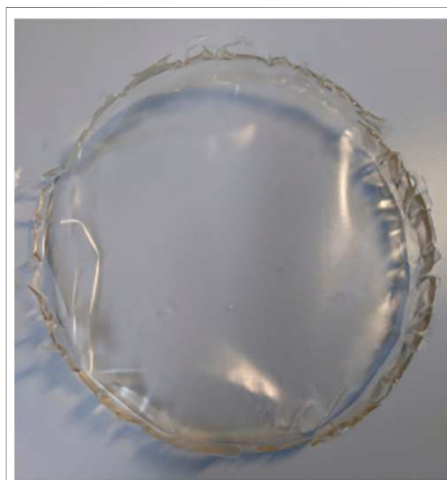
FIGURE 2 | A film with 1% BudMA and 30% C4ASA.
