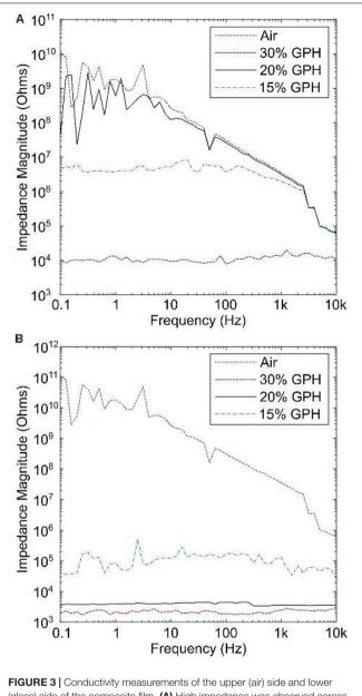
**FIGURE 3** Conductivity measurements of the upper (air) side and lower (glass) side of the composite film. (A) High impedance was observed across all concentrations of graphene, with the lowest observed in the 30% graphene polymer. (B) Measurements performed on the lower side of the polymer indicate that the resistance is several times lower, particularly for the 30% graphene polymer.
