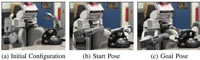
Fig. 5: Configurations for valve turning path.
