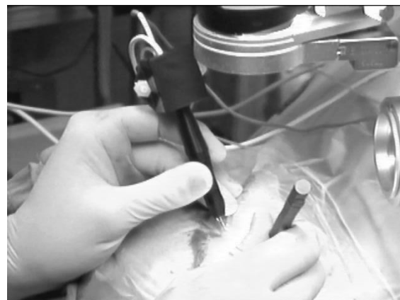
Fig. 3. Recording instrument motion during vitreoretinal microsurgery using inertial sensing. The 6-DOF sensing module, roughly cubical in shape, can be seen at the proximal end of the instrument in the left hand of the surgeon.
