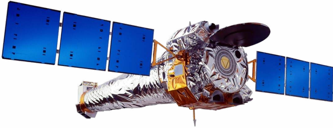
Figure 1. Illustration of NASA's Chandra X-ray Observatory in its operational configuration: 13.8-m length, 4.2-m diameter, 19.5-m wingspan, and 4800-kg (dry) mass. The Chandra flight system comprises the Telescope System (including the mirror assembly and optical bench—"tube"), the Spacecraft Module (surrounding the mirror assembly at one end of the optical bench), and the Integrated Science Instruments Module (containing two focal-plane detector arrays at the opposite end of the optical bench). [Credits: NGST]
