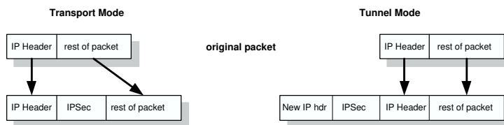
Figure 4.2: Transport mode and tunnel mode.
