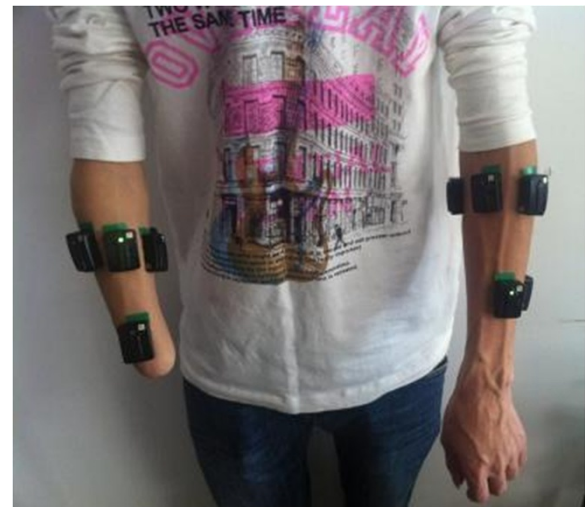
Figure 1 Electrode placement. Eight parallel-bar electrodes were placed on the skin surface of intact arm and amputated arm, respectively.
