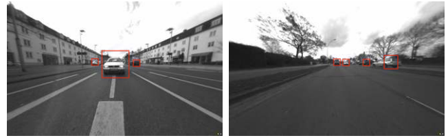
Fig. 11. Front and rear vehicles detection on the acquired images. In the right example, the image distortion affects the recognition of a vehicle.
