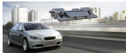
Fig. 10. The Bosch stereo video camera detects objects' height and distance as well as capturing standard video images.
