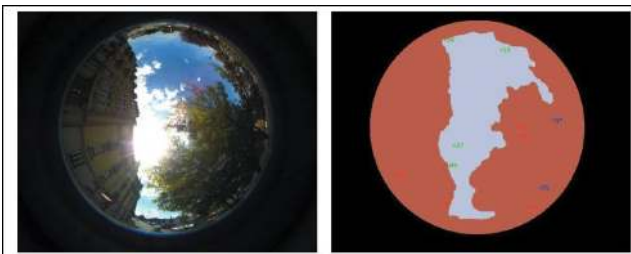
Fig. 4: Fish-eye image acquired on the top of a road vehicle and processed in order to detect masking and sky areas [43]
