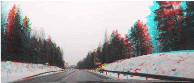
Fig. 5: Matching FAST features detected from consecutive images in good weather condition. Features shown using a red circle for the first image and yellow cross for the second.
