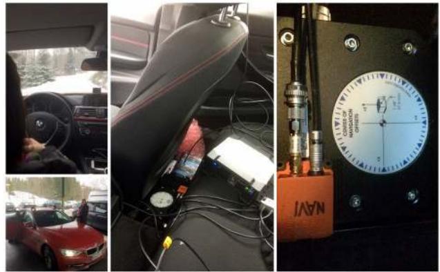
Fig. 3: Test equipment. Left up: GoPro camera on the wind shield, left down: antennas on the vehicle's roof. The hybrid receiver and the SPAN reference system were rigidly attached together (right) and located behind the passenger seat (middle)
