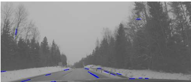
Fig. 6: Lines detected (blue) from the image using Hough Transform
