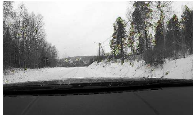
Fig. 8: FAST features detected and matched from two images taken in snowfall (the contrast has been increased to get the snowfall and water on the wind shield visible in the image)
