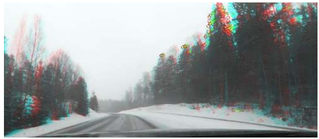
Fig. 7: Matching FAST features detected from consecutive images from snowy and icy road. Features shown using a red circle for the first image and yellow cross for the second.
