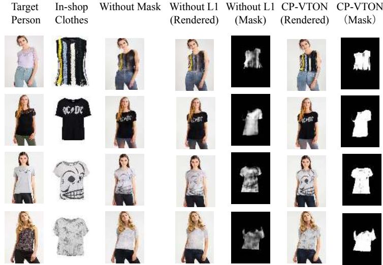
Fig. 7. Ablation studies on composition mask and mask L1 loss. Without mask composition, UNet cannot handle well even minor misalignment and produces undesirable try-on results. Without L1 regularization on mask, it tends to select UNet-rendered person, leading to blurry results as well.
