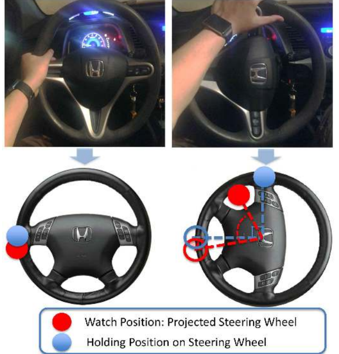
Figure 4: Holding position and the projected position of smart watch on steering wheel.
