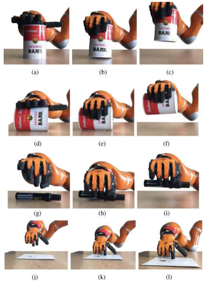
Fig. 15. Photosequences of tasks performed by SoftHand 2 mounted on a Kuka LWR. In (a, b, c) and (d, e, f), a same object is grasped from two different sides, achieving two different grasps. In (g, h, i), the robot performs a precision grasp, and in (j, k, l), it slides a paper through the use of the index finger.
