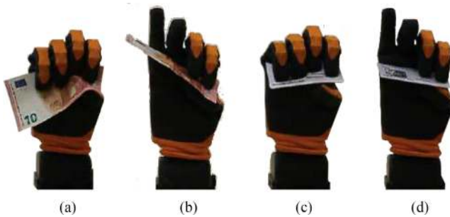
Fig. 14. Comparison of grasping capabilities, between one DoA and two DoAs. The grasps (a) and (c) are obtained using the first DoA of the SoftHand 2. The second DoA enables more natural grasps when grasping small and/or flat objects, as with the banknote and the credit card in panels (b) and (d). (a) Banknote. (b) Banknote. (c) Card. (d) Card.
