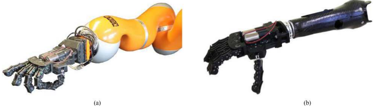
Fig. 8. Pisa/IIT SoftHand 2 presents a completely self-contained design, i.e., motors, sensors, and electronics are all on-board. This enables an easy integration in robotic manipulators. As an example, panel (a) shows SoftHand 2 mounted on Kuka LWR. Panel (b) shows instead the application of SoftHand 2 as a prosthesis. The hand is here integrated with a custom socket designed for sEMG prosthetics.
