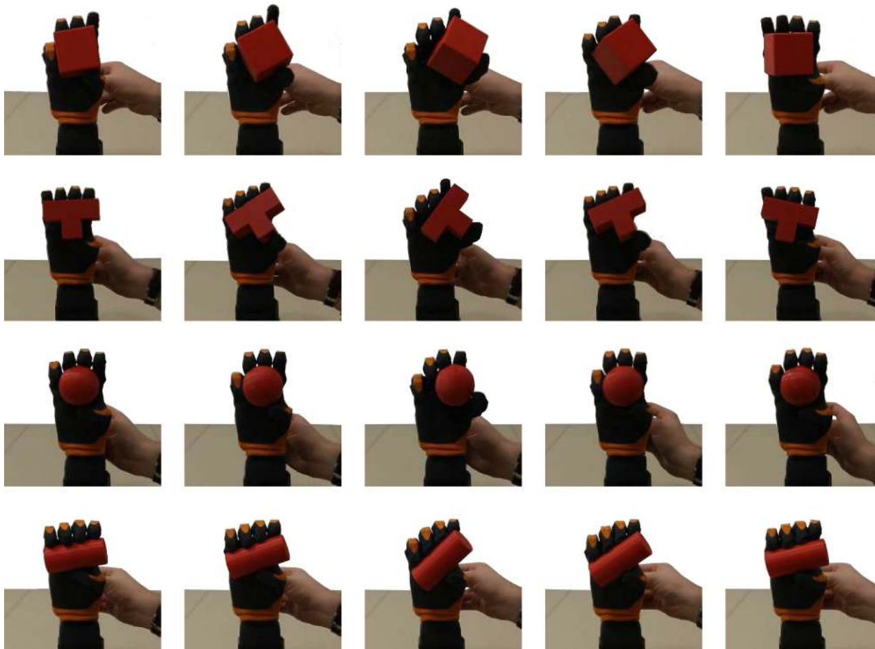
Fig. 19. Examples of in-hand manipulation. A same feedforward input allows to rotate objects with different shapes, relying on the intelligence embodied in the mechanism.
