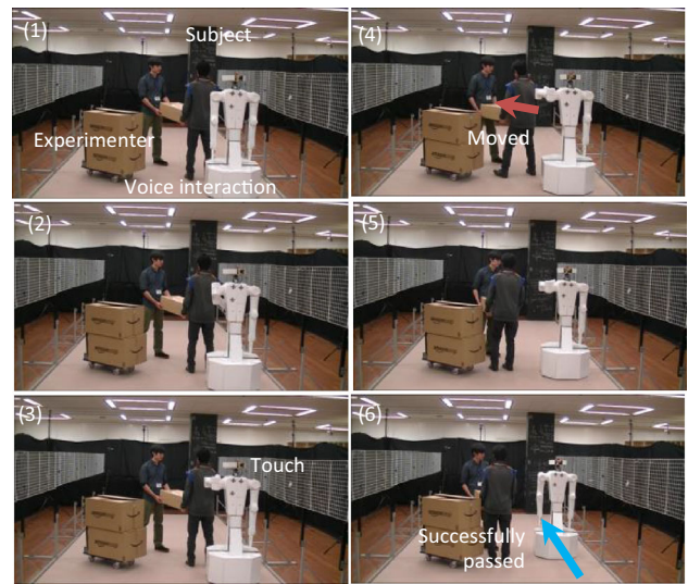
Fig. 19 Human and robot behaviors in static scenario ( HA = 0 ) for advanced experiment. Robot first used voice interaction and human did not move. Then, with IA function, robot used physical touch and successfully passed
