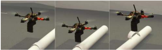
Fig. 10. Still images from a sample “swooping” trajectory using the vision-based controller developed in this paper. The background has been washed out slightly to improve visibility.
