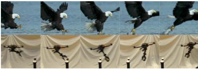
Fig. 2. Top: A bald eagle snatches a fish from the water [18]. Bottom: A quadrotor dynamically grasps at 3 m/s using a custom gripper [2].
