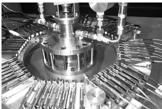
Figure 3 – Laboratory implementation of simulated in-cylinder conditions. The silica-walled pressure vessel (centre of picture) is shown configured for liquid fuel injection. Inlet and outlet hoses allow for purging and pressurization of the chamber with air or nitrogen. A heating element in the base of the chamber controls the temperature. The outer support ring is used for mounting and alignment of the 64 fiber optic elements, in 4 projections of 8 beams each.
