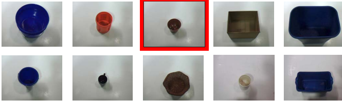
Fig. 8. The result of using a Nearest Neighbor classifier to label novel objects as ‘containers’ or ‘non-containers’. The flower pot (outlined in red) was the only misclassified object. Sparse coding features were extracted from the 10 training objects and used in the classification procedure.
