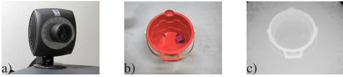
Fig. 1. The robot's vision system: a) the ZCam from 3DV Systems [11]; b) color image of the red bucket captured by the camera when mounted on the robot; c) the depth image corresponding to b).
