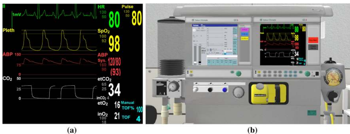
Fig. 2 Vital signs monitoring of the system. The screen of anesthesia simulation software (a) is captured for the respirator's right monitor (b)
