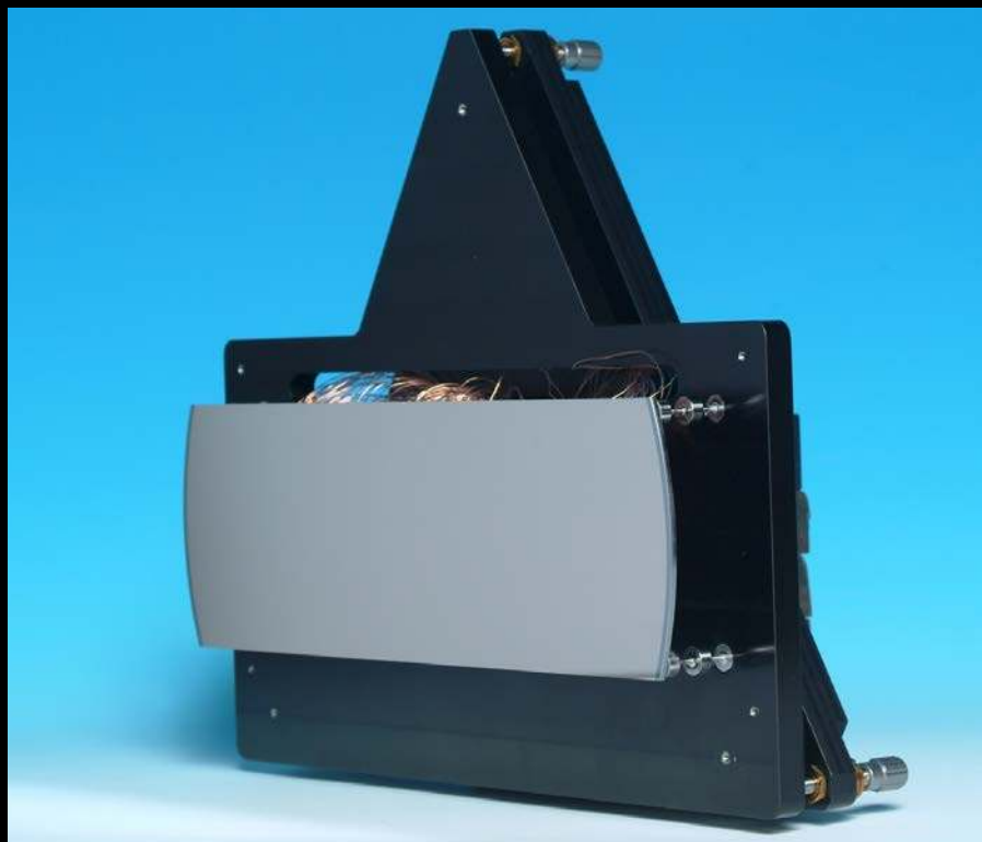
Xinetics deformable mirror (DM) uses 4 \times 27 array of electrostrictive (PMN) pads bonded to mirror. Xinetics and ANL characterized DM.
