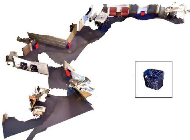
Fig. 1. On right: a discovered object (a trash bin) from two separate, partially overlapping maps (not shown) where one map had the object, while the other did not. The object was used to automatically tune a segmentation algorithm to segment other instances of the object in a new, unseen map (on left). The discovered objects are highlighted in red to show detections.
