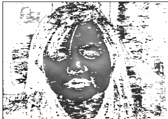
Figure 1. Example of the output of the Face Color Classifier. Dark areas are classified as skin-colored.
